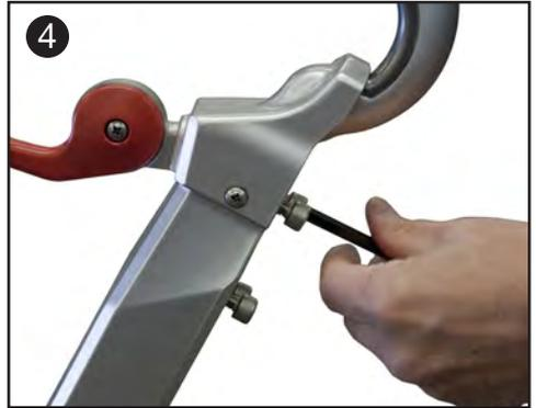
**Step 3:** Using a 6mm Allen wrench, and the four screws, assemble the Bottom Slide to the Handlebar Tube. Tighten firmly, making sure there is no gap between the Slide and the Handlebar Tube (Fig. 6).
