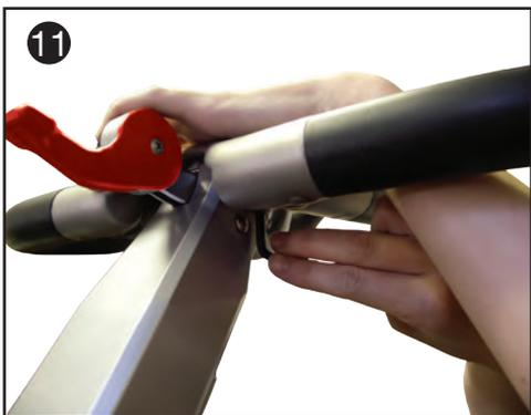
**Step 2:** Tilt the handlebar assembly slightly to place the socket head cap screws (M8x1.25 X 12 SS) into the mounting holes (Fig. 11). Once each screw has been started, place the palm of one hand on the center of the handlebar pressing firmly and evenly onto the handlebar post. With the other hand tighten each screw with the Allen wrench until the head of each screw just makes contact with each hole. Now tighten each screw evenly.
