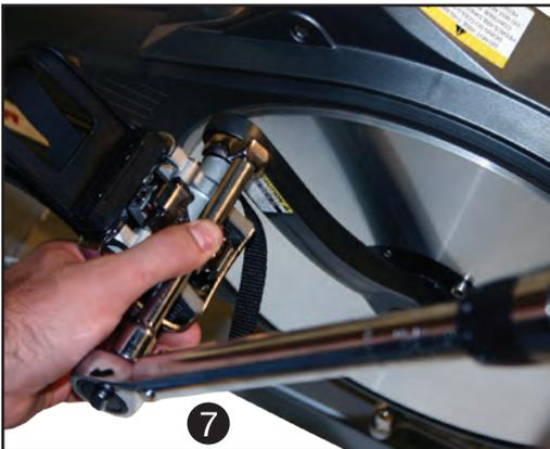
**Step 2:** With a clean cloth, wipe the threaded area of the pedals. Apply Loctite 242 to the pedal threads. Install the pedals into the crank arms, use the 15mm open-end wrench to tighten. Finish with the torque wrench, 15mm crowfoot, and 4" extension. Torque pedals to 45 Nm (35 ft-lbs) (Fig. 7).
